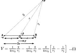
If  $(r, \theta)$  are polar coordinates of point P with respect to mid-point O of dipole, then By geometry,
