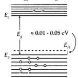
The expression for the conductivity of a p-type semiconductor: A p-type semiconductor has holes as the majority charge
