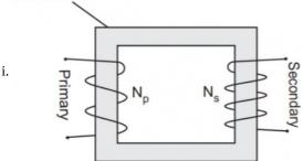
The working principle of transformer is mutual induction.
