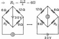
For the equivalent circuit. when the Wheatstone bridge is balanced, there will be no deflection in the galvanometer.
