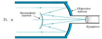
It consists for large concave (primary) paraboidal mirror having in its central part a hole. There is a small convex (secondary) mirror near the focus of concave mirror. Eye pieces if placed near the hole of the concave mirror.
